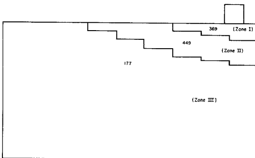
Fig. 9. Conceptual grid: conductances of horizontal elements ( \text{ohm}^{-1} ) (not to scale).
